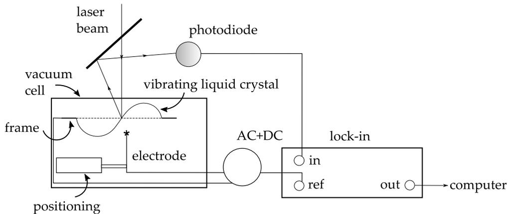
**Figure 5.** Experimental set-up for the vibrating liquid crystal. With the help of the photodiode we can measure the deviation of the laser beam from the starting direction. Figure reproduced from [10].
