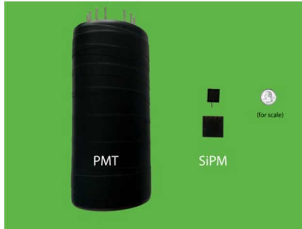
Figure 6. Size comparison of a PMT and a SiPM [15].
