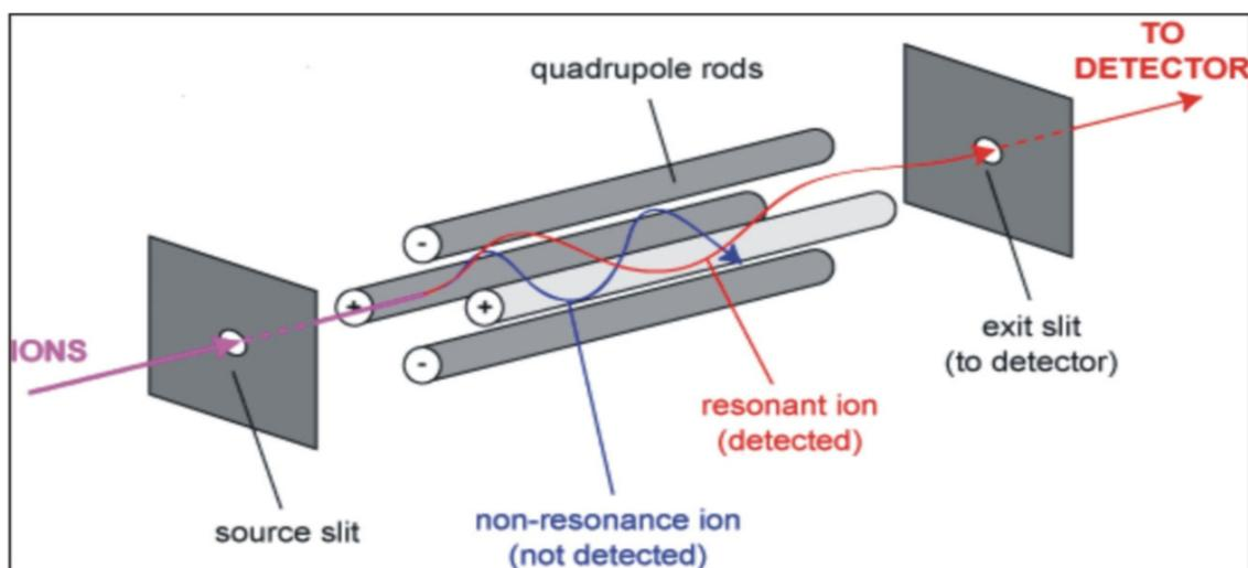
**Figure 5.** Schematic of a quadrupole mass separator (QMS), with represented trajectories of two ions with different mass-charge ratio [9].
