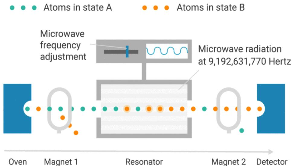
Figure 1. Schematic of caesium atomic clock [8].
