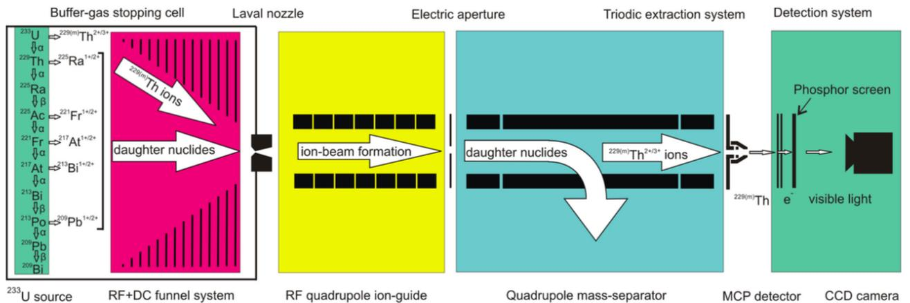
**Figure 6. Schematic of the experimental setup 2.** Reproduced from: *Direct detection of the  $^{229}Th$  nuclear clock transition*, *Nature* **533** (2016), 47–51.
