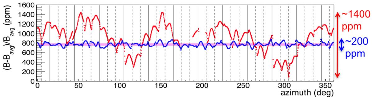
**Slika 10.** Azimuthal variation in magnetic field. The red curve indicates  $(B - B_{\text{avg}})/B_{\text{avg}}$  in October 2015, the blue in June 2016 and the pink band is the desired variation, which was achieved in August 2016. Reproduced with permission of W. Gohn (2016) [3].
