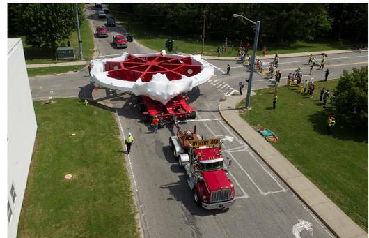
Slika 9. The Muon g-2 team successfully transported a 14-meters-wide electromagnet from Long Island, New York to the Chicago suburbs in one piece. The move took 35 days and traversed 5150 kilometres over land and sea. Reproduced from [9]. This image is in the public domain.
