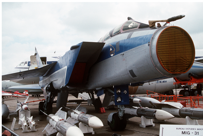
(a) PESA radar v nosu letala MiG-31. Vir: [13].
